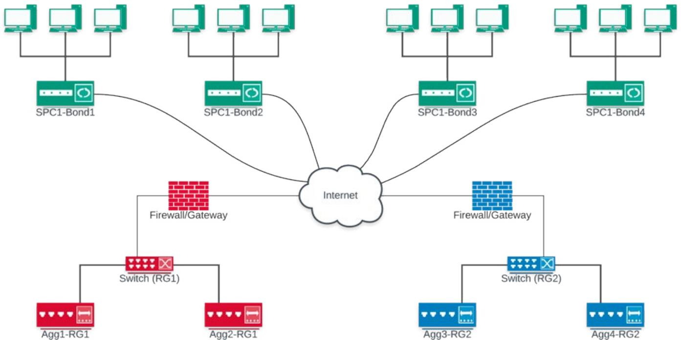
In the scenario shown in this diagram, data from customer site SPC1-Bond1, which is directly supported by Agg1-RG1, is being sent to customer site SPC1-Bond2, which is supported by Agg2-RG1.
