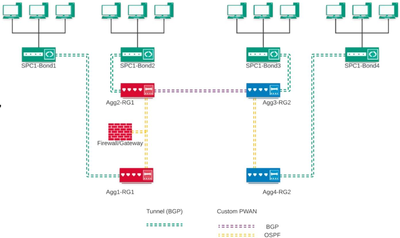
In this example, this particular routing could be set up to ensure data between RG1 and RG2 uses a specific network path between Agg2-RG1 and Agg3-RG2. This might be done to avoid more costly -- but faster -- routes that would be established using Managed Mesh.
