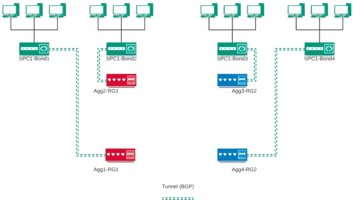
Using the same PWAN — but with OSPF and BGP manually configured to let selected Aggregators route traffic to each other, Agg1-RG1 can communicate with Agg2-RG1 and Agg2-RG1 can communicate with Agg3-RG2.
