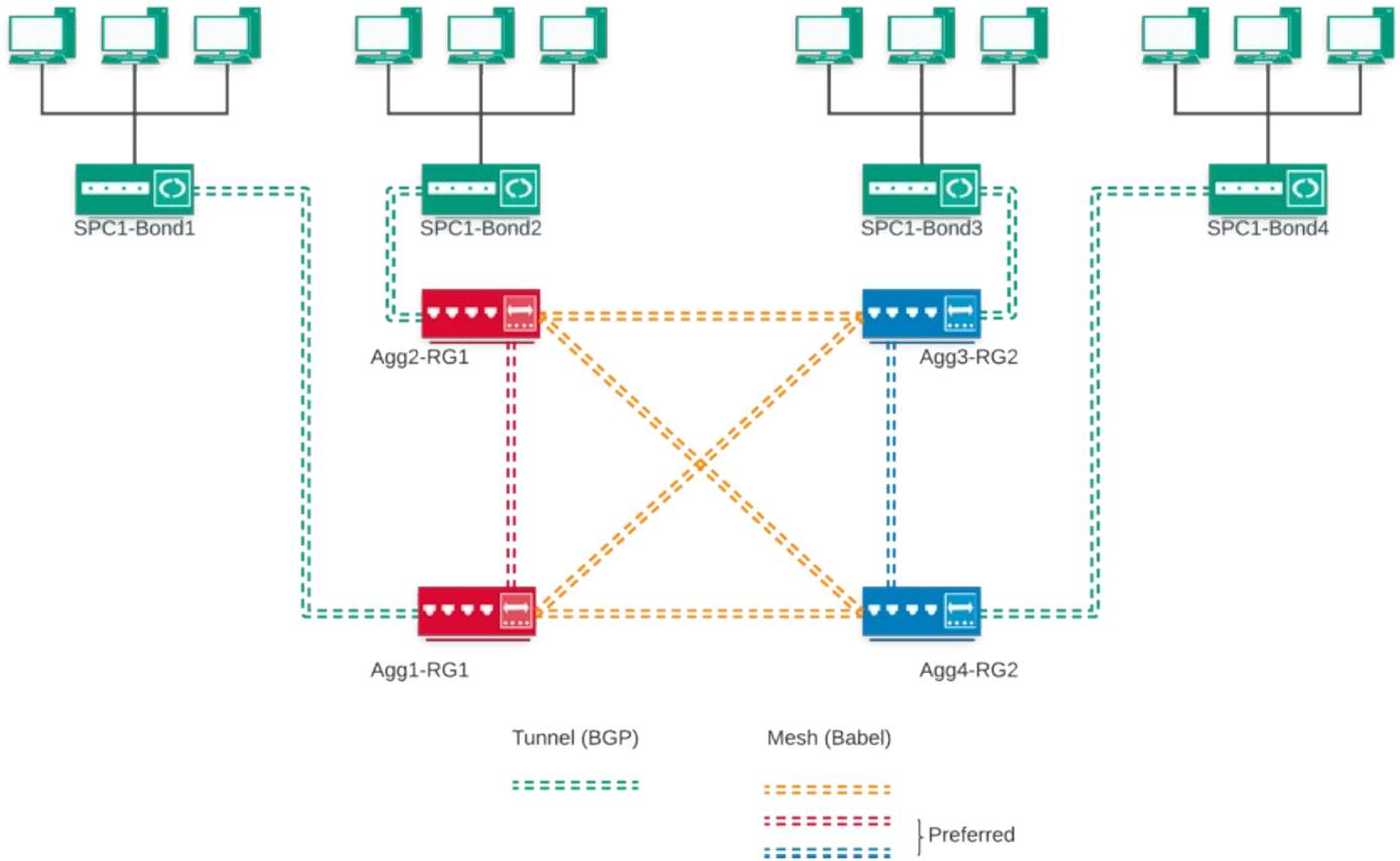
Turnium SD-WAN automatically creates meshed infrastructure for each specific customer space in which Managed Mesh is turned on in the Management Server. Managed Mesh is toggled on within a space's Private WAN settings. Once turned on, all Aggregators added to that space are automatically meshed.
