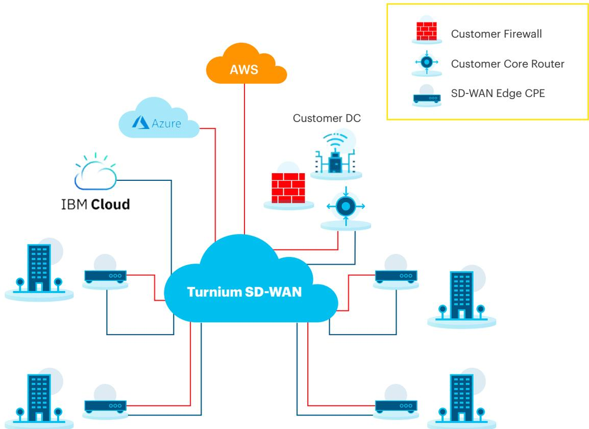
Turnium's core provides the networking between three of the four customer sites, as well as to the data center. A carrier private network is shown being integrated into this example, to illustrate how Turnum can deploy hybrid networks by integrating carrier-provided circuits in the SD-WAN.
