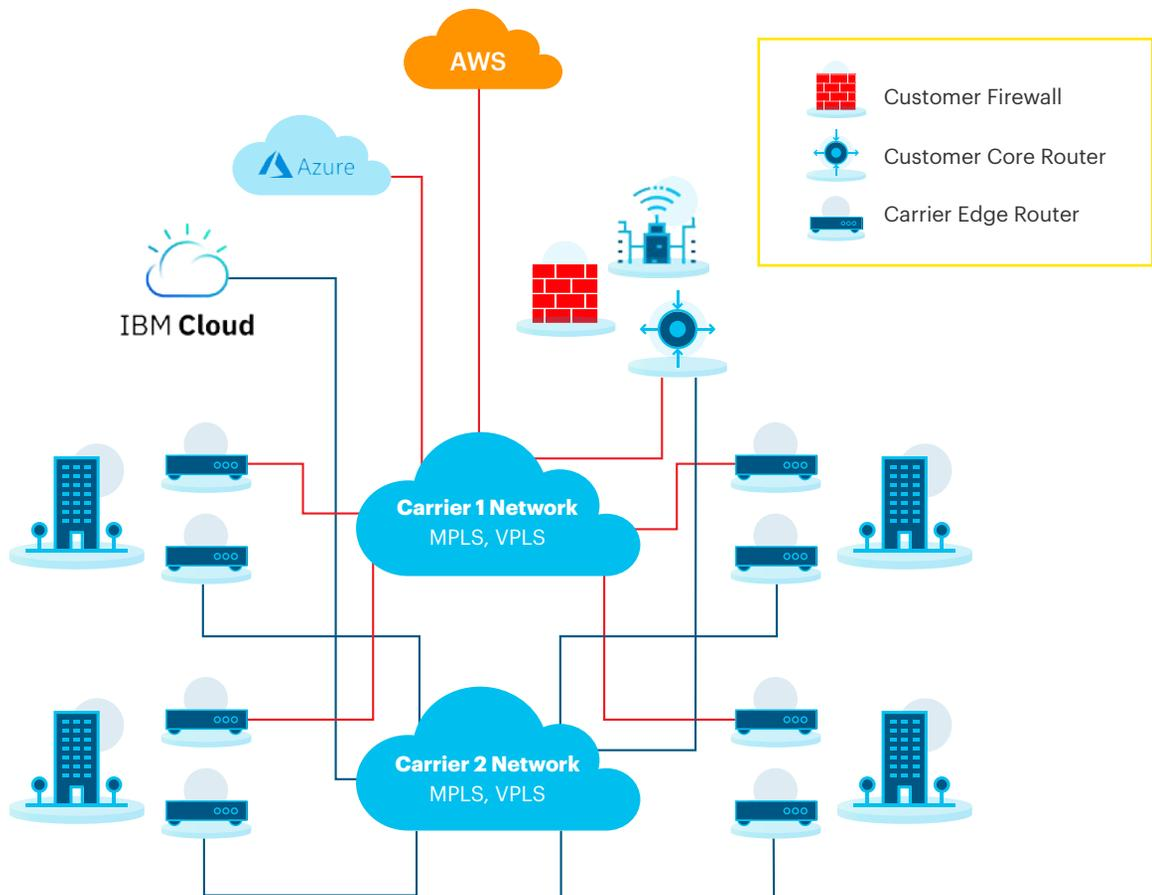
Packets are labelled to route traffic in the network based on pre-engineered destinations and paths making networks more static and harder to change.
